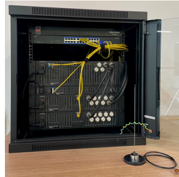
Fig. 1. SPARTAN™ RX rack with expansion and extension modules
