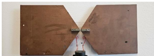
Figure 1. Spark gap switched wideband dipole antenna. 1
